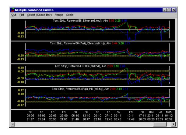
This example shows a mix of Kodak and Fuji E6 strip lots from a processor, looking just at the D-max and HD. This allows the user to examine the relationship between the different strip types and decide on optimum corrective actions.
