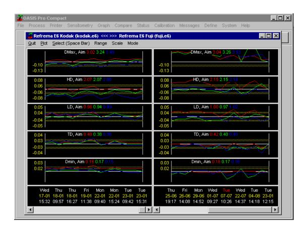
For optimum process control, processing of both Fuji and Kodak controls is recommended. No other process control program allows this type of comparison - you need to see both plots together to gain a full understanding of process changes.
